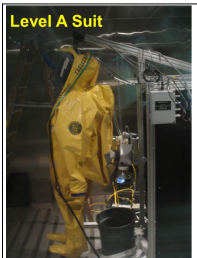
Figure 1. Sweating manikin testing of TDA's Hazmat suit cooling device at NIOSH
