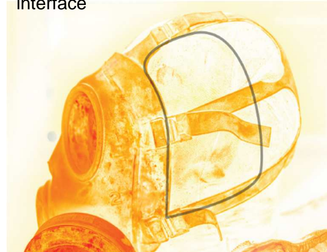
Leakage through the prototype gasmask-hood interface
